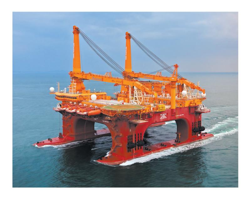
The SSCV OOS Gretha is a large, state-of-the-art, multi-functional, dynamically positioned construction semi-submersible crane vessel and accommodation unit. It has a sizeable hotel capacity up to the highest standards.
