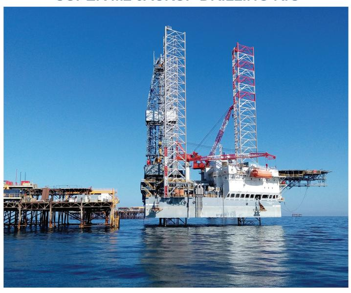
Caspian Driller, the Super M2 jackup drilling rig is designed for all year benign conditions in accordance with ABS assessment criteria. It is based on the F&G L780 Mod II jackup design.
