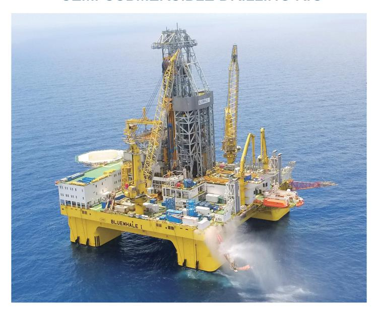
'Bluewhale I' is an ultra deepwater drilling unit built by CIMC Raffles. It is able to operate in water depth of 3,658m, and drilling depth up to 15,250m. It is designed with dual hoisting tower and facilities with DP3 system and preliminary mooring position system. It will provide accommodation for 200 POB and can operate in 95% deepwater areas all over the world, including the Gulf of Mexico, West Africa, South Atlantic, Asia, Australia etc.
