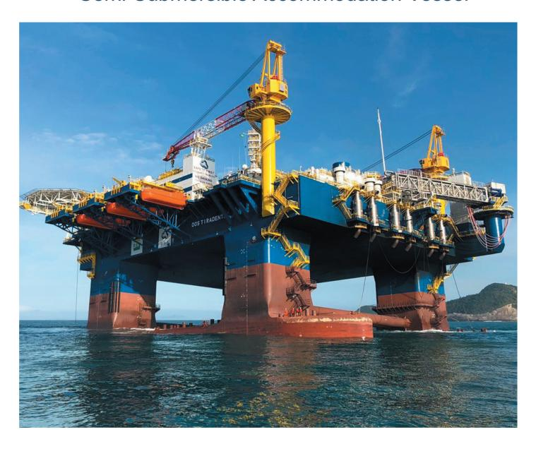
CR600 'OOS Tiradentes' is a Column Stabilized Semi-submersible Accommodation Rig, Featuring the latest technology, the CR600 design accommodation semi-submersible rig is capable of operating gangway connected in deep water and in harsh environments alongside fixed platforms, floating platforms and Floating Production and Offloading vessels, with a full complement of deck cranes and fire-fighting capabilities.
